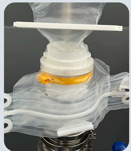
4. QuickTric complete installation with Flecozip secondary housing
